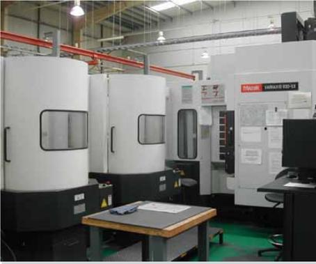
Bromford's flexible manufacturing system (FMS) is built around a 5-axis MAZAK Variaxis 630 machining center
